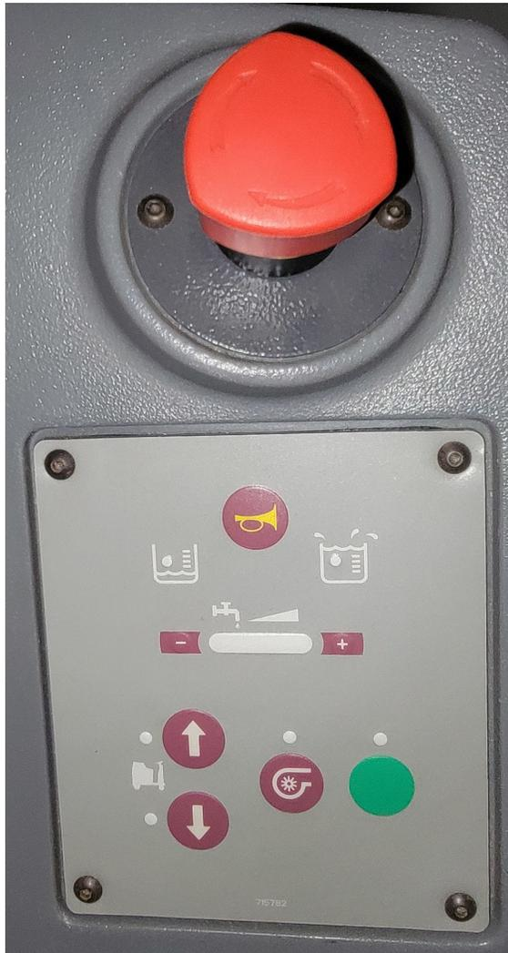
There are two E-Stop switches on Roboscrub 20, one located at the front of the machine by the Control Panel and one at the back of the machine by the Beacon.
