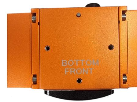
Front IFM Camera is Labeled TOP and BOTTOM. Care should be taken that it is installed correctly
