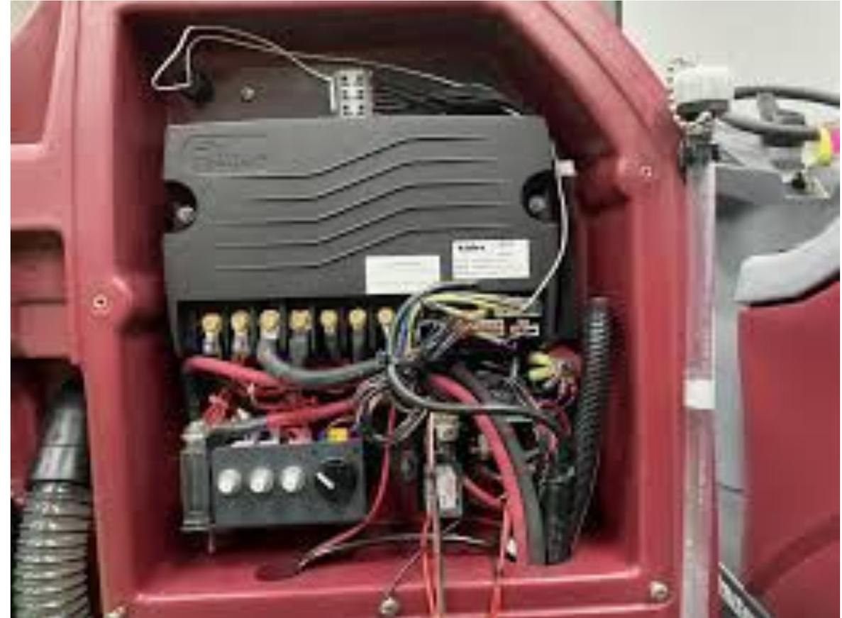
When the Kinetek controller software detects an error condition, it will shut down the operation of the controller and provide a visual indication of the error code via the red LED, flashing in a Hexadecimal format.
