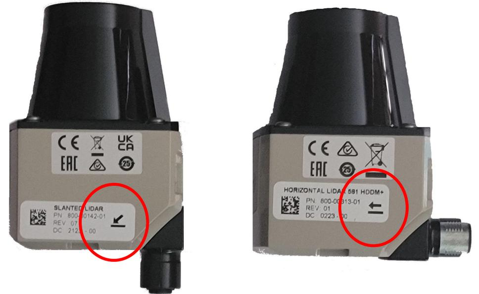
LiDARs are shipped with the M12 connectors in the position shown on the Right. The connectors can be rotated 90° to the use position as shown on the Left
