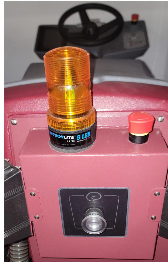
The Start/Pause Button is located on the back of the RoboScrub20
